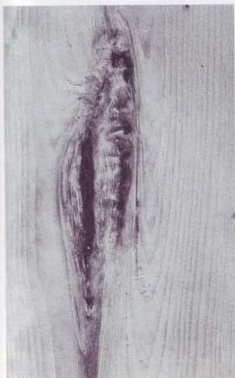
Pockets: Caused by damage to the cambial (tree growth) layer, repaired by the tree with bark or pitch.
